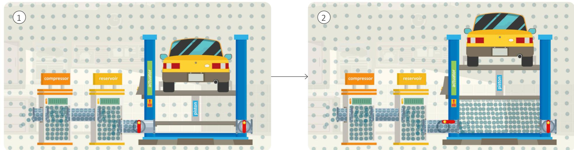
Air is sucked from the atmosphere and squashed in a compressor. The compressed air is stored under high pressure in a reservoir. When the in valve between the reservoir and the actuator is closed, air cannot move out of the reservoir and the piston remains down.
